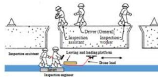
Figure 3 Pattern diagram of inspection work by drone
