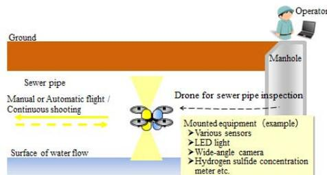
Figure 1 Diagram of inspection with a drone
