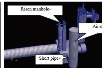
Figure 5 Countermeasure 2 (Case3): Intermediary Manhole Attachment
