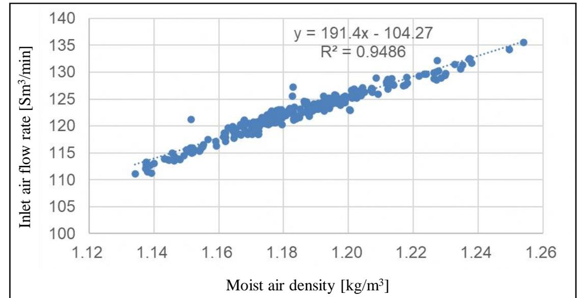
The relationship of the maximum inlet air flow rate with the moist air density (right) has less variation than that of the inlet temperature (left). This means using moist air density can accurately reflect changes in the blowers' operating performance better.
