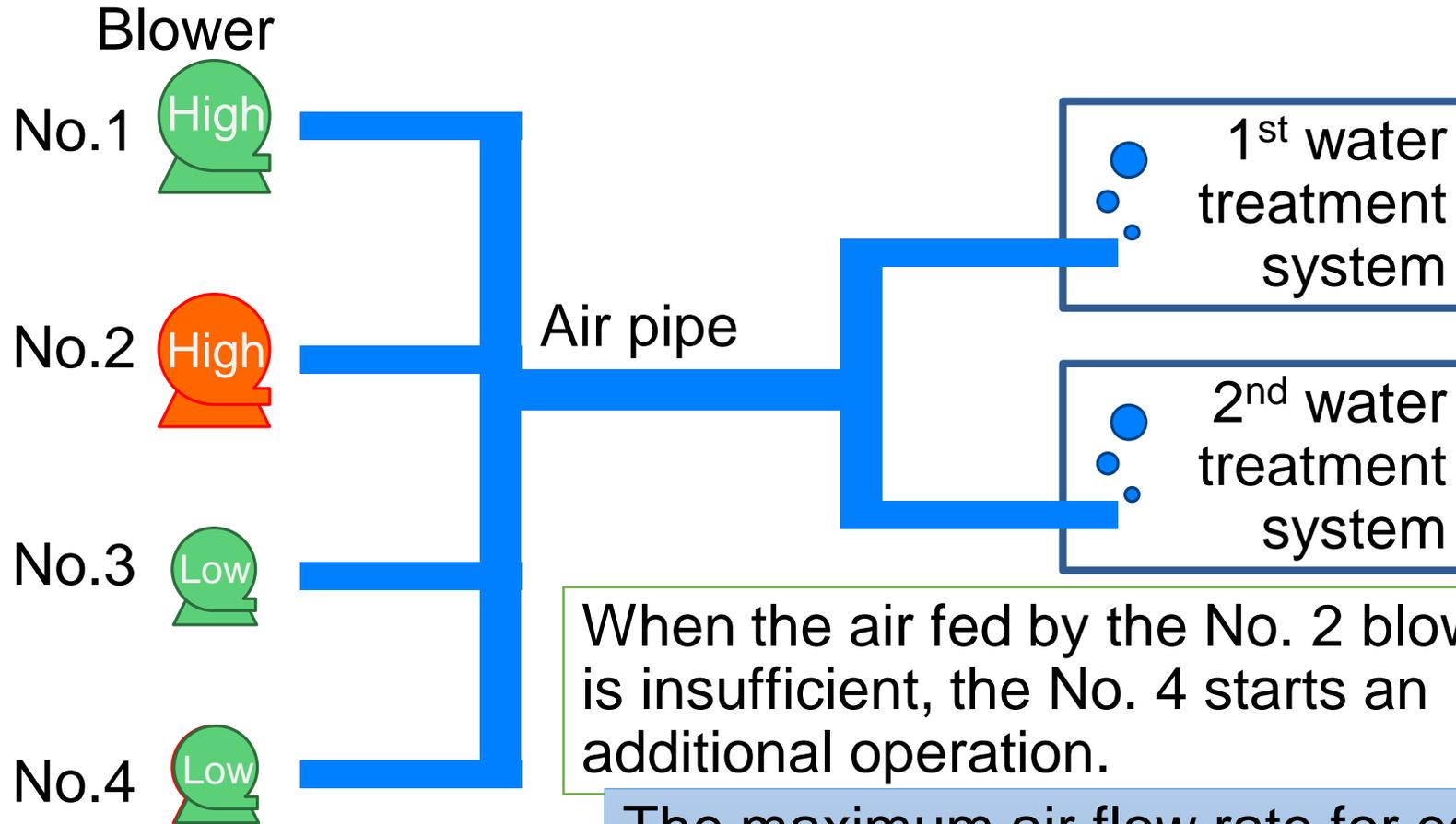
When the air fed by the No. 2 blower is insufficient, the No. 4 starts an additional operation.
