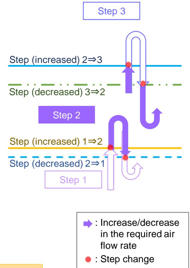
It was confirmed that the settings for step 1 to 2 and step 2 to 3 can work in the overall temperature range.
